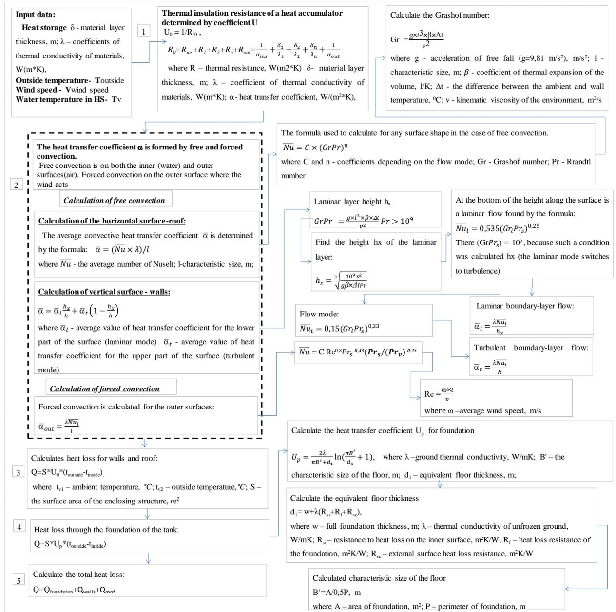
**Figure 3.** Heat loss calculation methodology [22]–[25]
