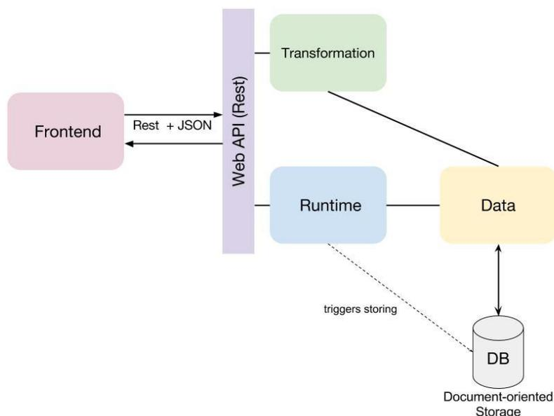
**Figure 4.** UeberFlow implementation components
